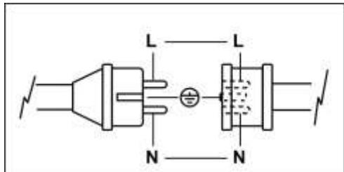
A models may be connected to a room thermostat **or** other accessories (such as the timer) by connecting to the thermostat plug (10).
